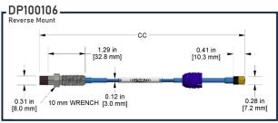
Lengths AA, BB, and CC are configurable in the CTC Part Creator
