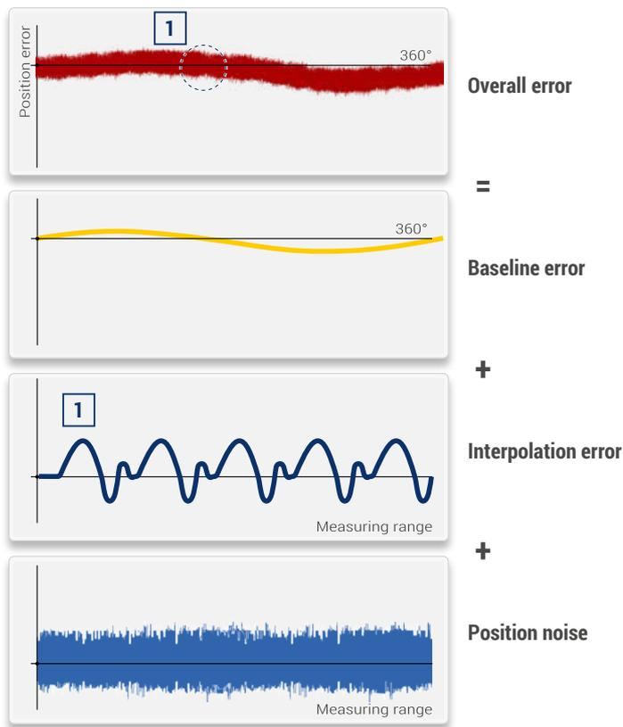
The accuracy of an encoder is mainly determined by the baseline error of the scale unit, the interpolation error of the optoelectronic scanning and the position noise.
