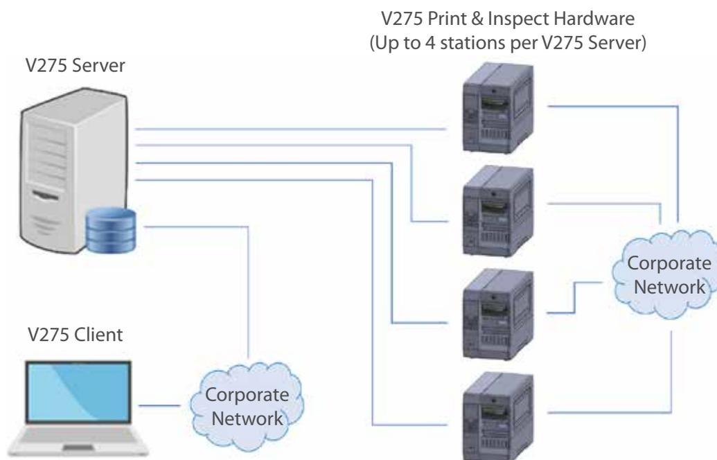
The V275 system architecture is designed to allow the flexibility to locate the V275 Server component in a central location, while accessing and controlling the system from any computer with a web browser and authorized access. It eliminates the need to have a server computer located next to every print & inspect hardware unit.
